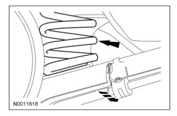
3. *NOTICE:* Tighten the new suspension fasteners while the suspension is at curb height or bushing damage and incorrect clamp load may occur.
