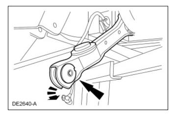
15. Lower the axle housing from the vehicle.
